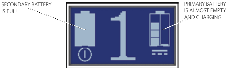
Figure 15. This display shows that two batteries are inserted. It also shows that the unit is connected to a power source. The secondary (left) battery is fully charged. The primary (right) battery is nearly empty and charging.
