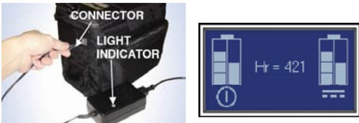
Figure 6. Connecting the power cord to the connector located under the Velcro flap. A typical battery charging screen is shown on the right
